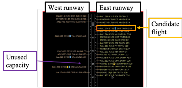
Fig. 8. Unused capacity on the West runway early in the bank.
